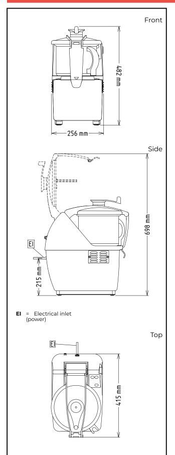
Electric Supply voltage: 600450 (DK55YVV) 200-240 V/1N ph/50/60 Hz Electrical power max.: 1.3 kW **Total Watts:** 1.3 kW Capacity: Performance (up to): 2.5 kg/Cycle Capacity: 5.5 litres Key Information: External dimensions, 256 mm Width: External dimensions, Depth: 415 mm External dimensions, Height:
